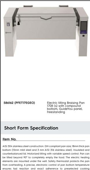
ensures fast reaction and exact adherence to preselected cooking temperatures between 50° and 250°C. TOUCH control panel. SOFT function. Possibility to store recipes in single or multiphase cooking process, with different temperature settings. Built in temperature sensors for precise control of cooking process. IPX6 water resistant. Configuration: wall mounted.
